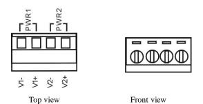
IT-ES716-IM-2GS-P( $12\sim48$ VDC) top panel provided 4 bit industrial terminal block, power input is 24VDC( $12\sim48$ VDC), the sign of the terminal block is V1-, V1+, V2-, V2+, it is redundant power input, both of them are  $12\sim48$ VDC.
